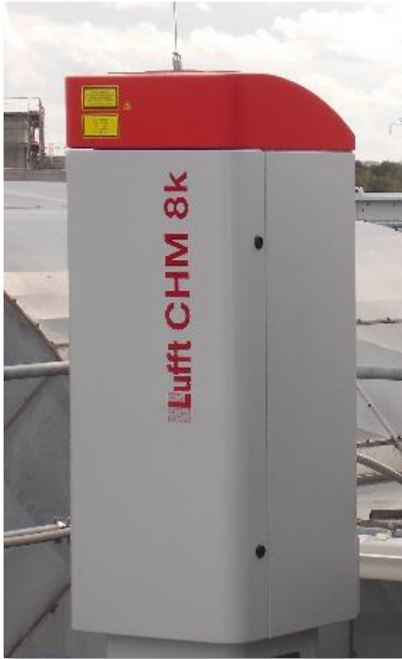
The Lufft CHM8k measures, amongst others, cloud layers in up to 8km heights
